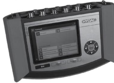
The HMG 4000 hand-held measuring unit is a portable measuring and data logging device. It was mainly developed for all values measured in relation with hydraulic systems, such as pressure, temperature, flow rate and position. Moreover, it provides a very high flexibility, even when it comes to evaluating other measuring values. The main applications are servicing, maintenance or test rigs.
